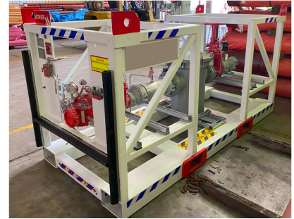
Engineered valve assembly skid
